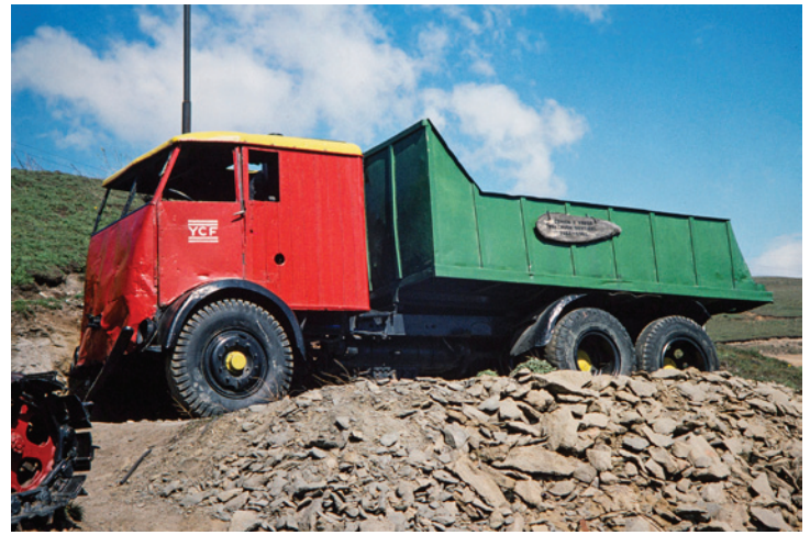
Only 1% remain of the original 100-truck order. This photograph taken by Fred M. Springer in 1996 shows a profile view of the three-axle steam-powered sentinel. The boiler sits behind the front axle between the frame and stoker-fed coal. The plaque on the dump bed says this truck operated from 1951-1961.
