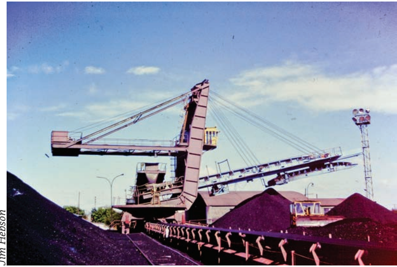
Contrast of old and new. At the coal terminal of Rio Gallegos, YCF operated a relatively-modern coal transfer system to create stockpiles of coal from which ships would be loaded. This equipment is still in operation today.
