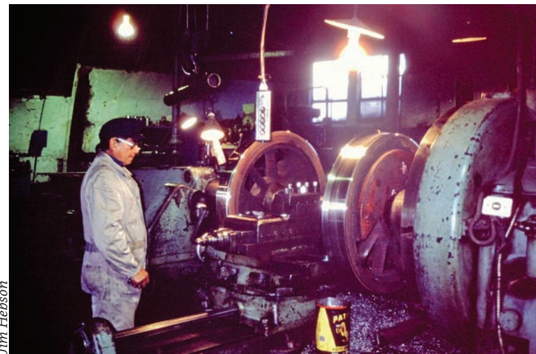
Turning driving wheels is a practice still performed on all manner of rail equipment to maintain a proper profile. In this photo, the machinist has already reprofiled the driver tires and appears to be surfacing the axle.
