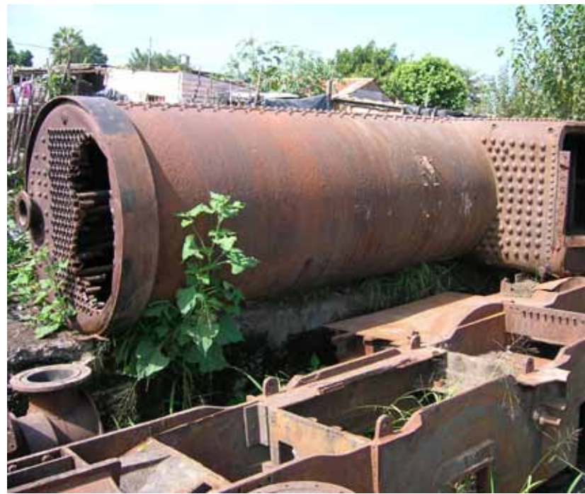
Forlorn and Vandalized This picture from 2010 shows the current state of "Argentina." While it is a sad sight, the view provides a clear look at the frame and tube arrangement of the locomotive.
