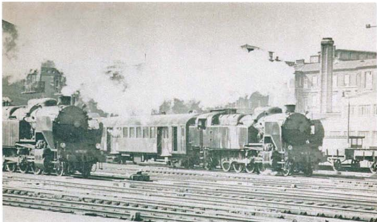
Suburban trains out of Gare du Nord, Paris, are worked by 72 2-8-2T's.
