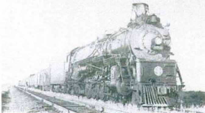
AFTER running 105 mph, Santa Fe poppet-valve 4-8-4 3752, dynamometer car 29, and Second 7, the Fast Mail, take siding just east of Dodge City, Kans., in May 1948 to clear the eastbound El Capitan. The performance delighted a North German Lloyd Steamship Lines engineering officer who was an observer on the dynamometer car during test.
