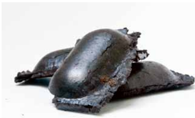
ABOVE - A view of the larger fuel pieces made in the newly-acquired pelletizing machine at NRRI's COLERAINE ENERGY LAB.
