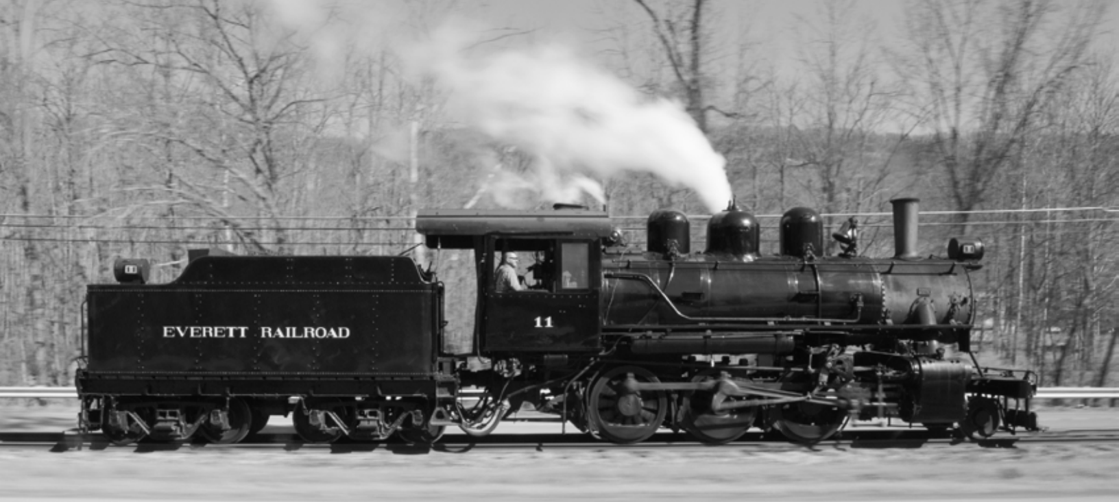
ABOVE - Everett Railroad No. 11 will serve as the testbed for the next scale of tests, thanks to the generosity of the railroad. This photograph, by Oren B. Helbok, nicely shows the scale of this standard gauge 2-6-0.
