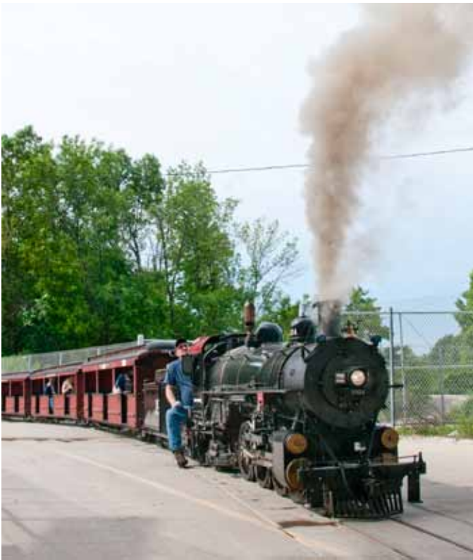
ABOVE - This was the darkest the smoke became during these tests, shown here just in preparation to depart the servicing facility. The small particle size lead to a very tight packing of the fuel, promoting smoke.
